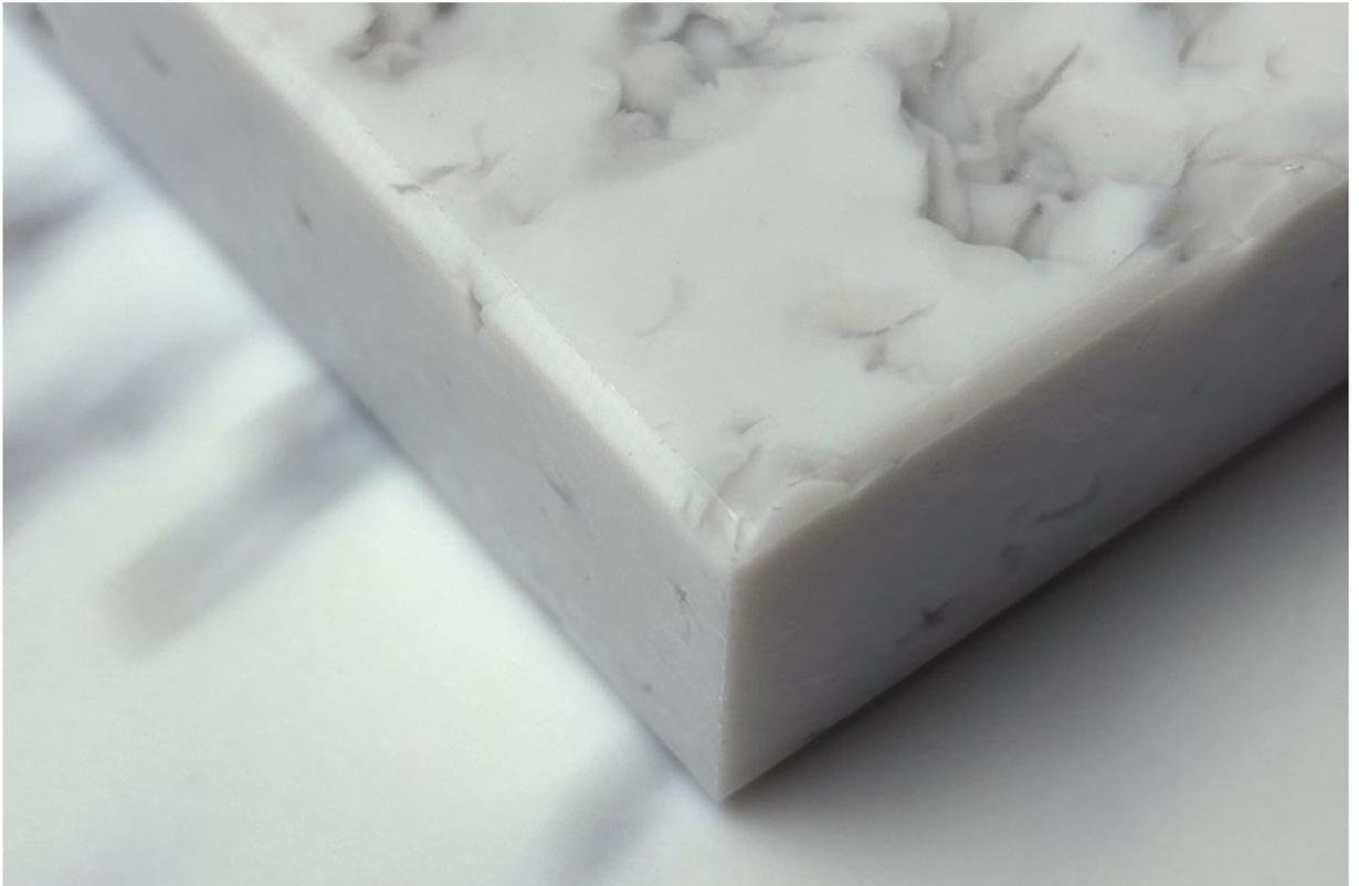
Untreated surface with rough sawn edge and 45° corner milling, panel design [Mica]
